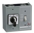
Manual Starter, fractional horsepower, duplex, 16A, 1 pole, 1 HP at 277VAC, toggle and selector, green indicator, NEMA 1
